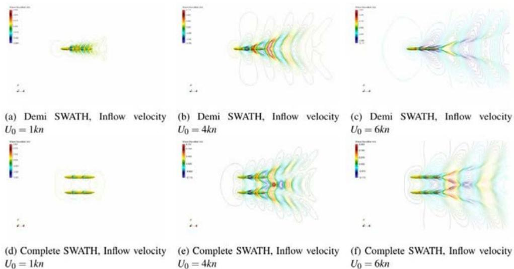
Fig. 6. Wave patterns comparison for the demi and complete SWATH configurations.
