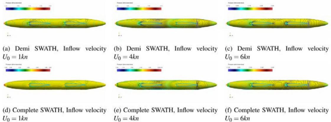
Fig. 5. Surface iso-pressure contours for the demi and complete SWATH configurations.
