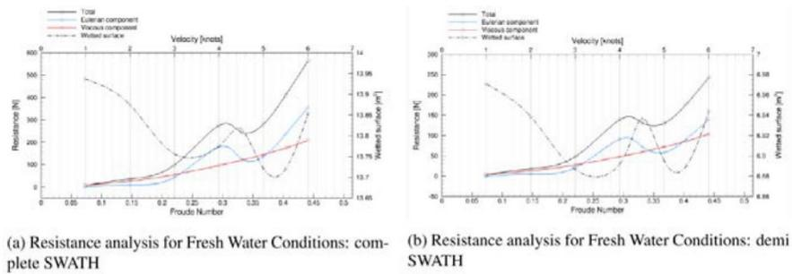
Fig. 3. Resistance analysis for Fresh Water Conditions: complete and demi SWATH.
