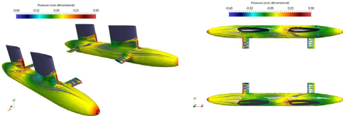
Fig. 7. Swath in fully appended configuration. Limiting streamlines colored with surface pressure.
