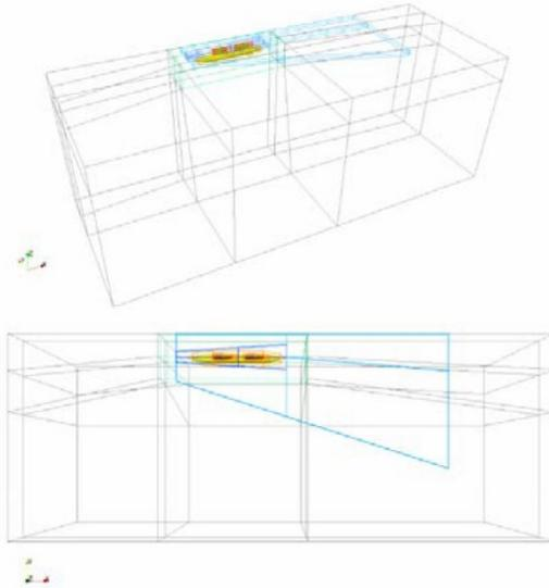
Fig. 2. Topology overview: black far background, light green near background, light blue free surface, orange hull, red struts.
