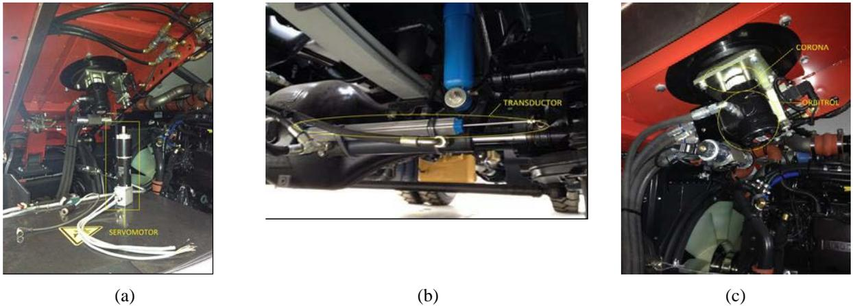
Fig 2 (a) Servo motor, (b) Steering transducer, (c) Orbitrol detail.
