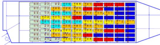
Fig. 11. Genetic algorithm result on a ninety location hold, stowed with ninety different rolltrailers, with six different destination ports. Destination port is coded by rolltrailer colour, showing no unload blockage is produced.
