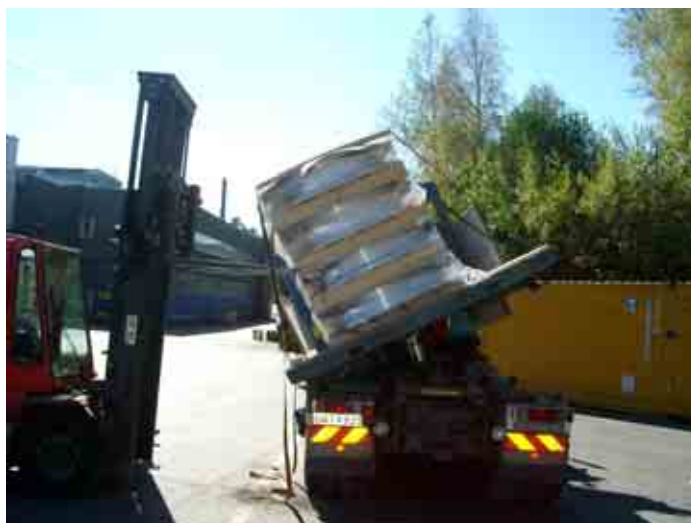
Test of securing arrangement for road transport.
