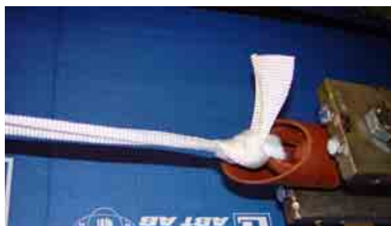
Test with webbing tied to fitting C.
