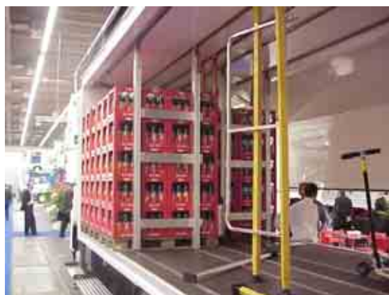
Cargo shifting device that can block 15 tonnes of cargo from shifting at a force of 0.8×g.
