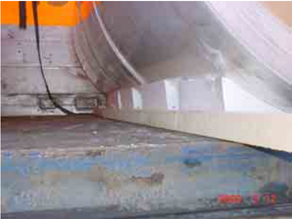
2 nd test – frigit scotches (soft) before the test
