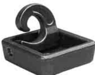
Forged securing fittings to be fitted in the side beam, front wall or container wall. The strength is guaranteed when wiggled: 20 – 55° towards the vertical plane. Weight 1.2 kg.
