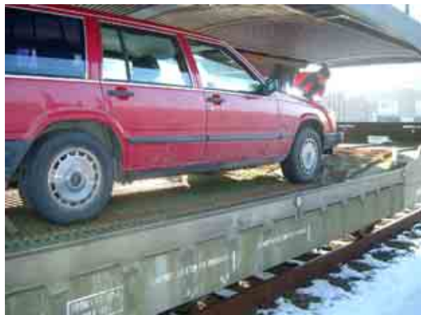
Volvo 740 with lashings in towing eyelet and tow hook. Scotchies were not in contact with the wheels (only precaution).
