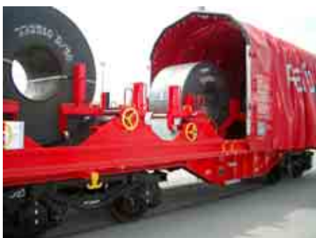
Cradles for coils with adjustable blocking arms
