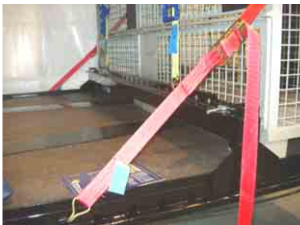
Blocking bar in combination with spring lashings.
