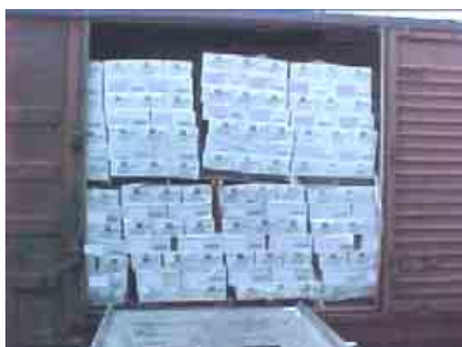
Damage due to insufficient strength of stretch/shrink-foil.
