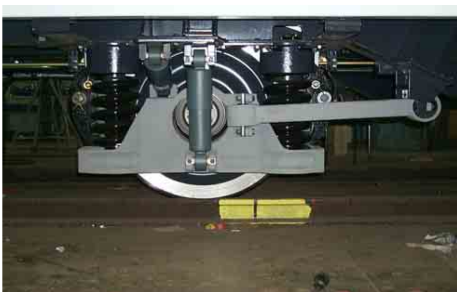
Wheel suspension for 25 ton axleload.
