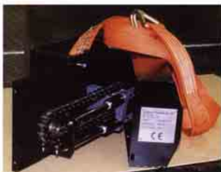
Here is a picture of the automatic pre-tensioner. It consists of 3 gas driven springs together with a chain that via a gear constantly keeps the lashing tightened.
