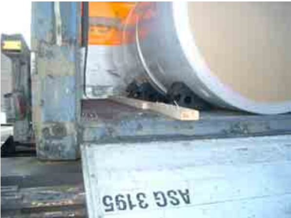
3 rd test – Rubber scotches + nailed batten
