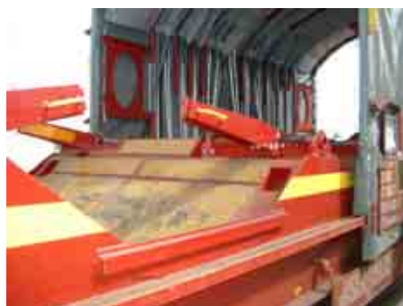
Cradles for coils with adjustable blocking arms
