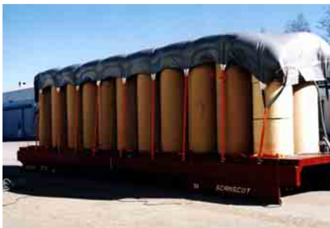
Airbag used to secure paper reels loaded on a cassette.
