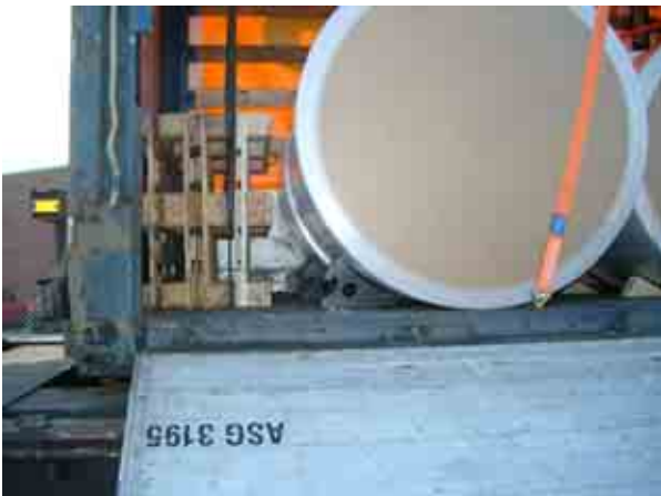
4 th test – Rubber scotches without batten
