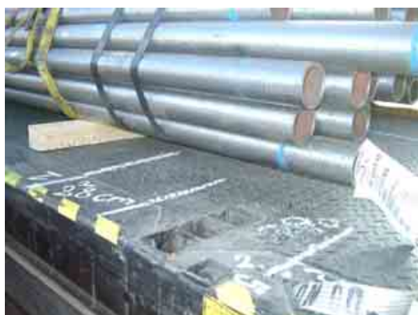
Section secured by indirect fastenings after the 2 nd test
