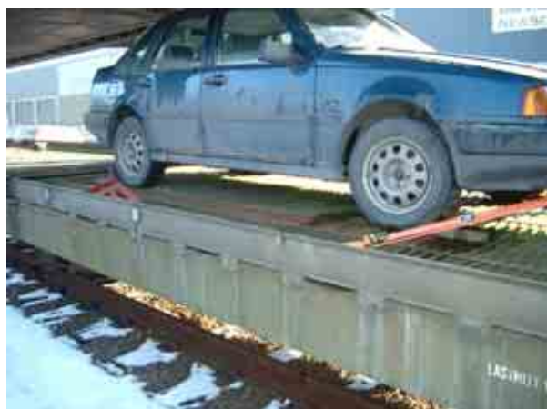
Volvo 440 secured with one scotch per wheel.
