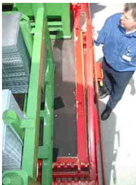
Stanchion possible to move sideways and to fold in to the floor.
