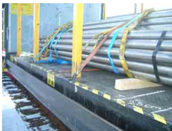
Section secured by two loop lashing pairs
