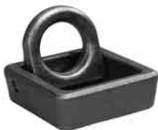
Forged securing fittings to be fitted in the side beam, front wall or container wall. The strength is guaranteed when wiggled: 20 – 55° towards the vertical plane. Weight 1.2 kg.
