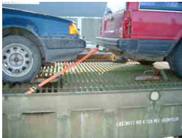
Volvo 740 with lashings in towing eyelet and tow hook. Volvo 440 secured with one scotch per wheel.
