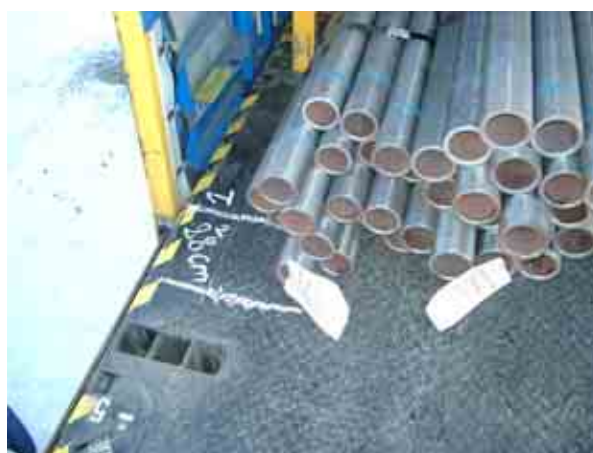
Section secured by indirect fastenings after the 1 st test
