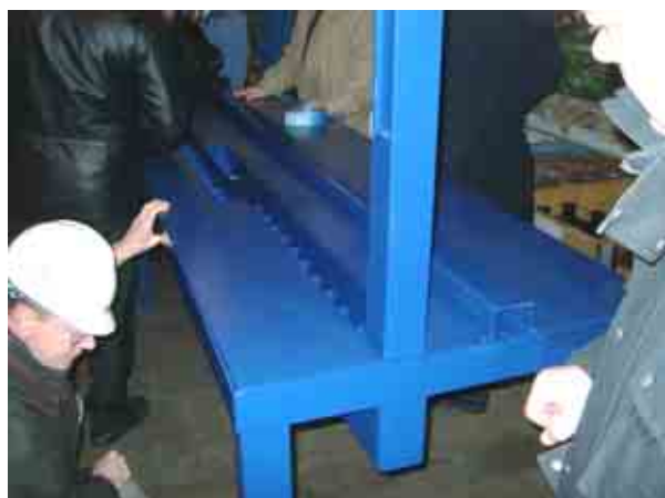
The prototype with raised stanchions and bolster.
