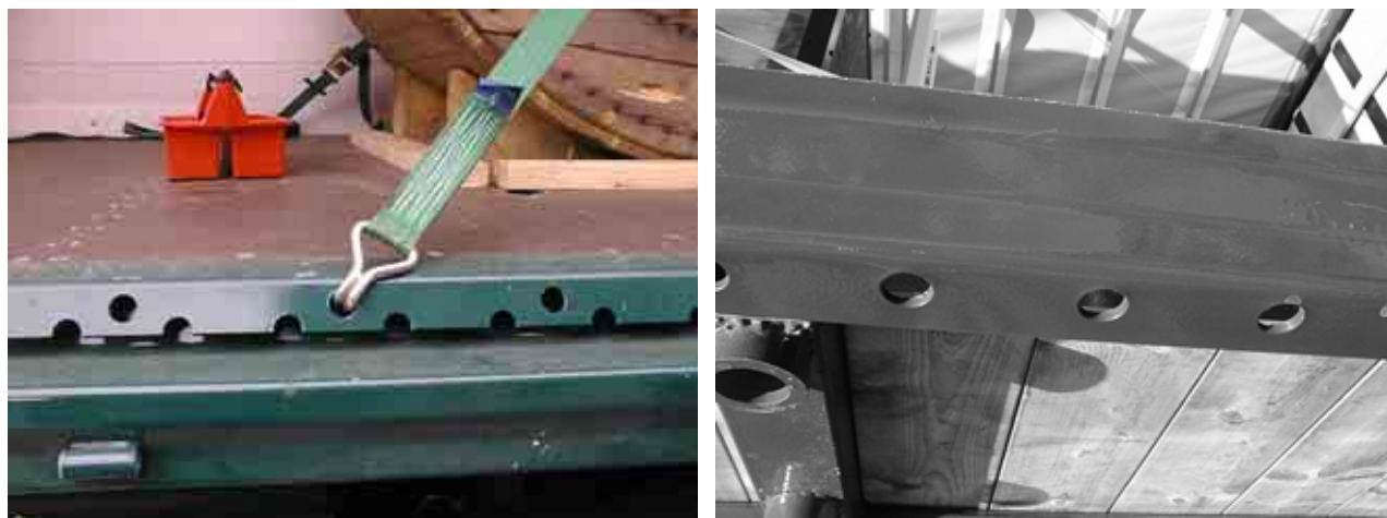
Side beam adapted for flexible lashings on the inside as well as on the outside of the sideboard. The pictures above show the side beam seen from the side and from underneath.
