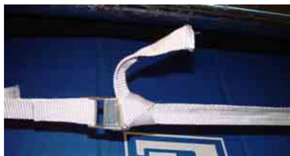
Test with SJ-lashing with clove hitch at the cam lock.
