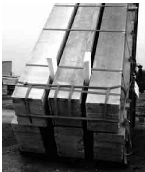
Test with elements of concrete secured with a spring lashing consisting of a round sling and four transverse lashing sewn into it.
