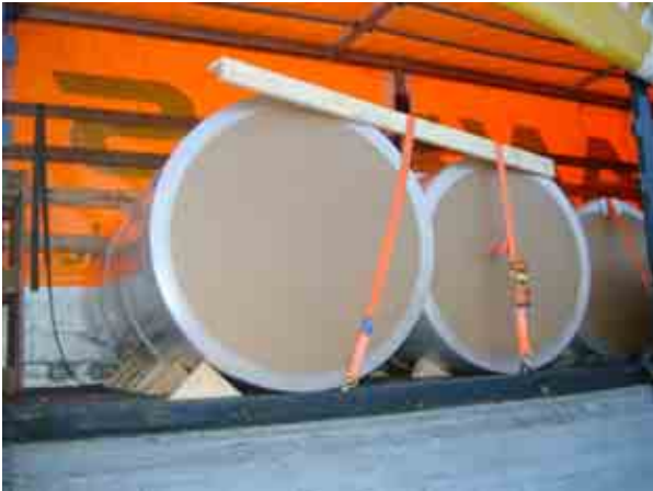
1 th test – nailed wooden scotches
