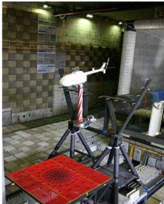
Figure 2: Acoustic test set-up with model helicopter & microphone array
