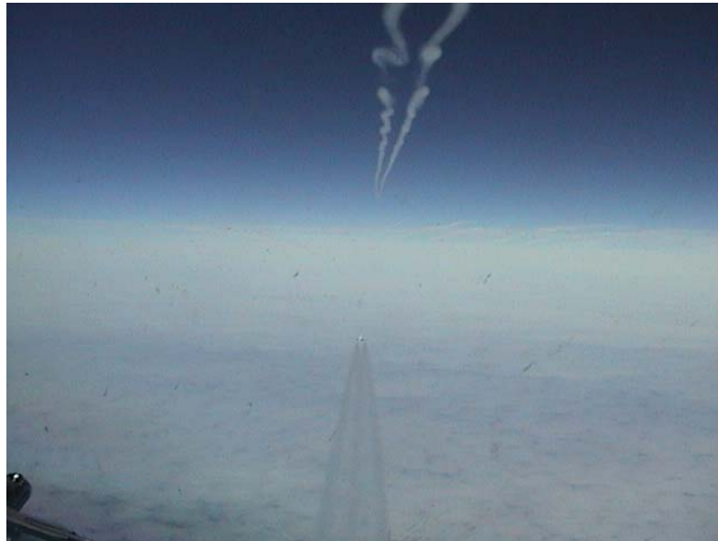
Figure 11-2: Crow instability as observed behind a Boeing 747 at cruise altitude (FL350) estimated to be at about 9 nm behind the aircraft. This instability manifests itself as an oscillation in the vortices leading finally to a 'connection' and the formation of vortex rings. (Courtesy of Arun Karwal, test pilot NLR).
