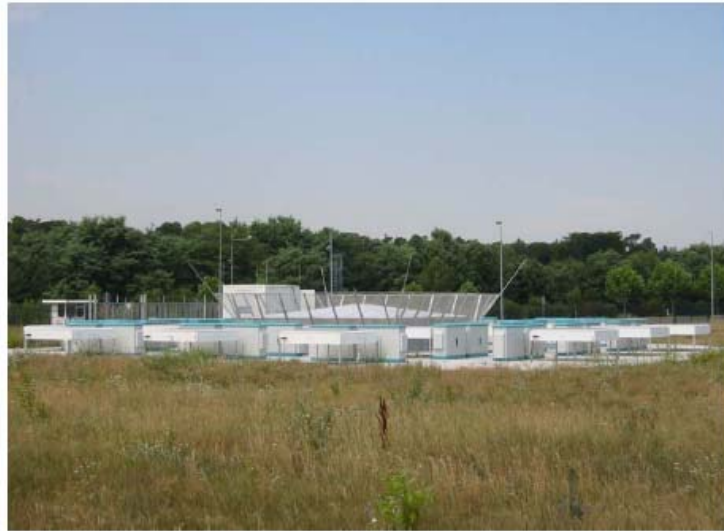
Figure 2-5: The Wind Temperature Radar (WTR) as installed at Frankfurt Airport intended to be used for the WSWS. The system provides wind velocity and temperature up till 1500 m height by combining Doppler-Radar for clear air measurements and Radio Acoustic Sound System (RASS) for measurements in bad weather.
