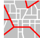
Strategic network too sparse. Although minimising route length, not so efficient as a connective network.
