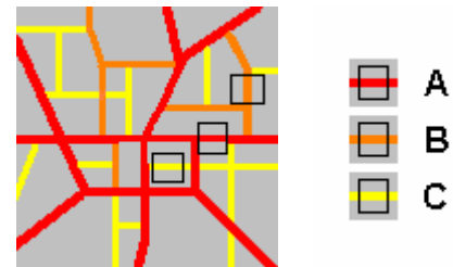
A three level 'hierarchy' based on link function. The levels could represent, for example, city roads (A), district roads (B) and local roads (C).
