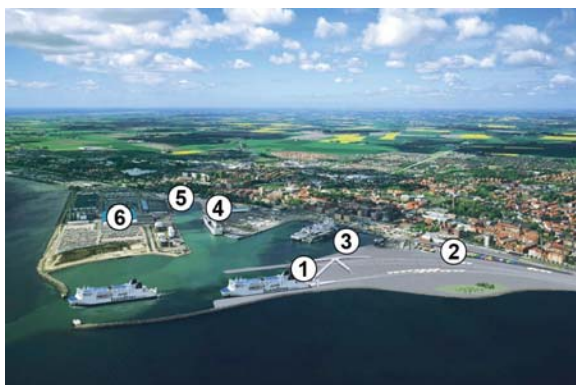
Picture 28: Trelleborg VISION 2005 includes (1) two new railway roro-berths, (2) a new intermodal terminal, (3) a new roro-berth, (4) extension of the check-in area roro terminal 1 (5) a new roro-terminal 2, (6) a new logistics centre
