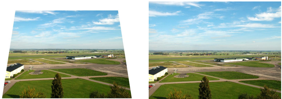
Figure 5 Perspective effects, before (left) and after (right) correction
