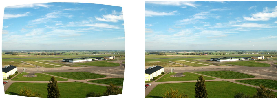
Figure 6 Barrel distortion, before (left) and after (right) correction
