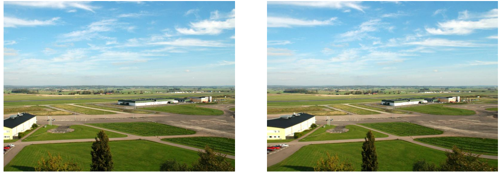
Figure 7 Geometrical correction from flat (left) to circular (right)
