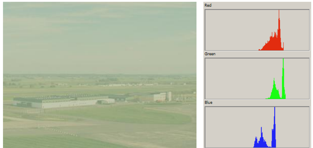
Figure 14 An example of unnatural colour balance, histogram to the right
