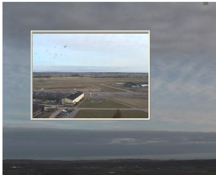
Figure 18 PTZ camera inlay on top of static camera
