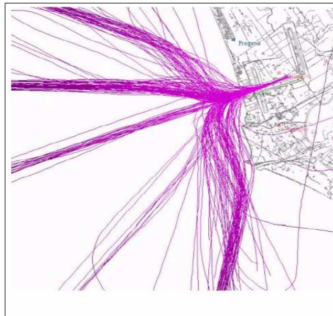
FIGURE 5 - Recorded Radar Tracks Implied by Take-Off Flights in Fiumicino ATZ.
