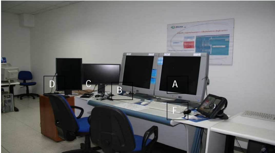
Figure 25. The executive and planner working position used during the simulation. The display were as follow: planner 2D radar display (A), executive 2D radar display (B), executive 3D radar display (C), and finally executive navigation display (D), see text for description. In front of the controller(F) was also placed the input device for the Instantaneous Self Assessment Tool for workload measurement.
