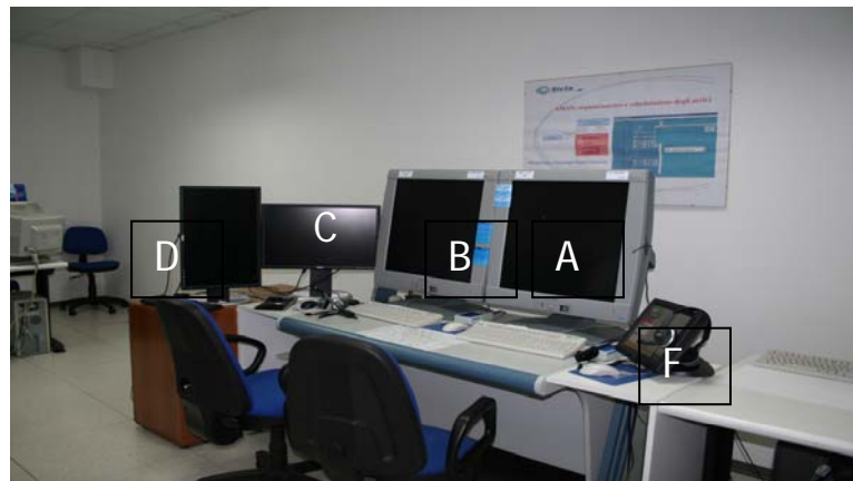
Figure 7. The executive and planner working position used during the simulation. The display were as follow: planner 2D radar display (A), executive 2D radar display (B), executive 3D radar display (C), and finally executive navigation display (D), see text for description. In front of the controller (F) was also placed the input device for the Instantaneous Self Assessment Tool for workload measurement.
