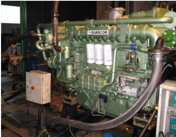
WP5 Figure 4: Guascor SF180TA 18 L diesel engine used in ethanol blend studies.
