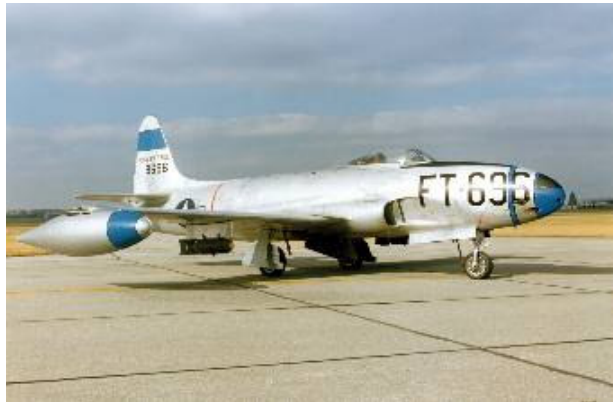
Fig. 2. Lockheed F-80C: complete magnesium construction
