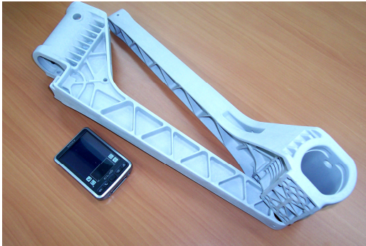
Fig. 7. Magnesium (AM50) die-cast helicopter components (IAI, Israel)
