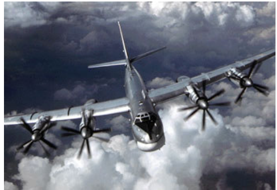
Fig. 4. TU-95MS: 1550 kg of magnesium
