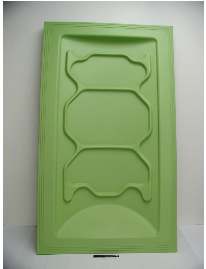
Fig. 8. Back panel of aircraft door pretreated by Gardobond ® X4729 and painted (AZ31B, superplastic forming by AMTS, Israel)
