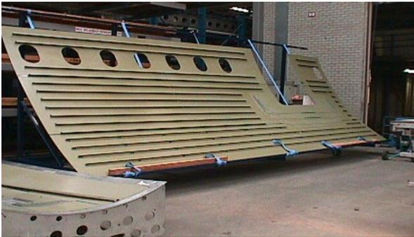
Figure 7: GLARE® fuselage panel
