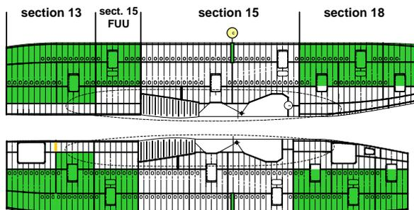
Figure 2: GLARE<sup>®</sup> (green) application at Airbus A380 [11]
