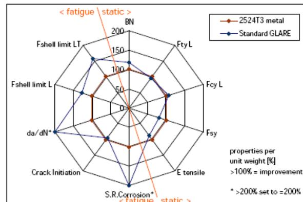
Figure 3: Improved properties of GLARE<sup>®</sup> in comparison to 2524 T3
