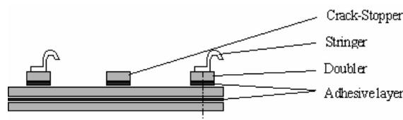
Figure 4: Design principle of Metal Laminates
