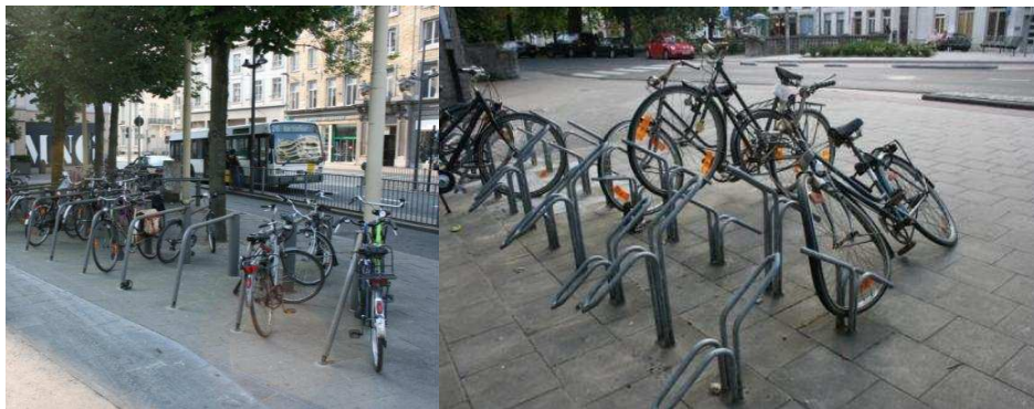
Pictures – recommended U-shaped bars and to be avoided paper-clip racks – T. Asperges
