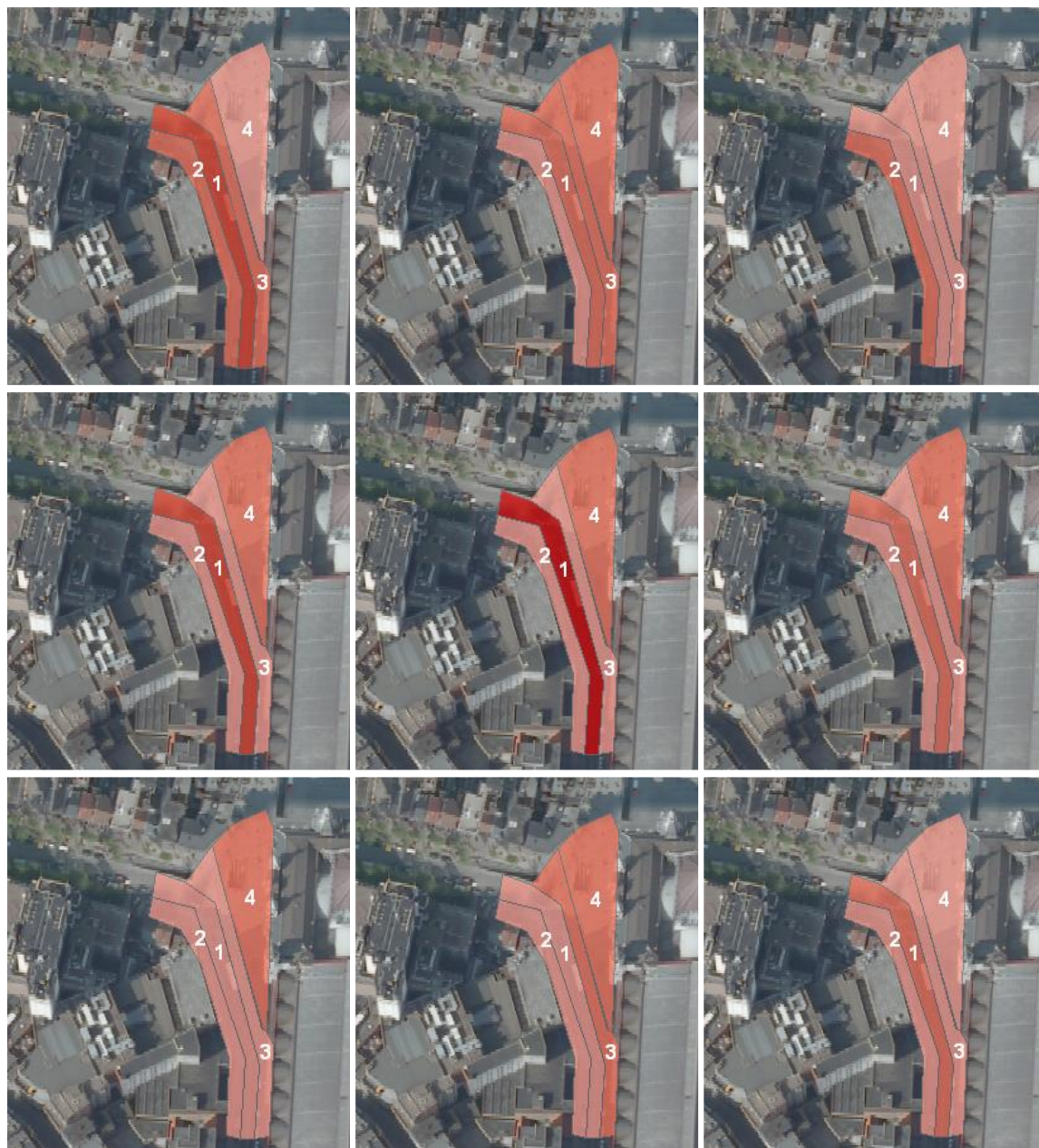
Figure 8: Mixture maps for the station area of Antwerp. Every map is a snap shot with a time difference of approximately 5 minutes. The colour value increases with increasing density.
