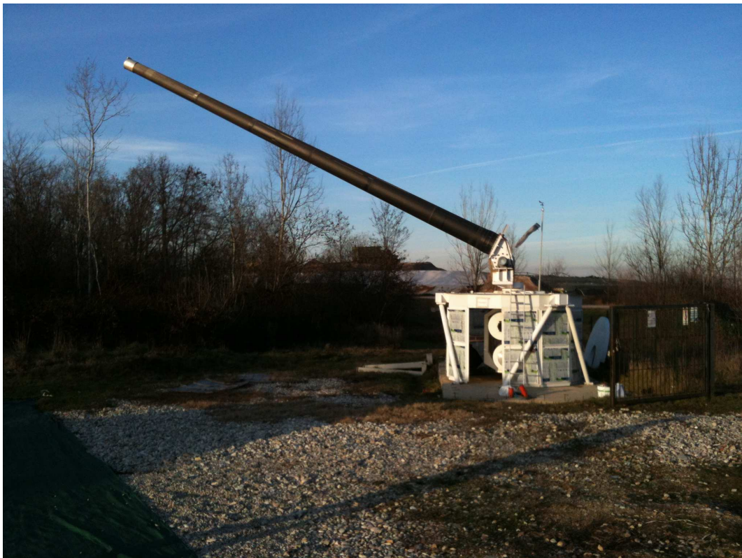
Fig. 10 The KitVes generator assembled for on shore tests
