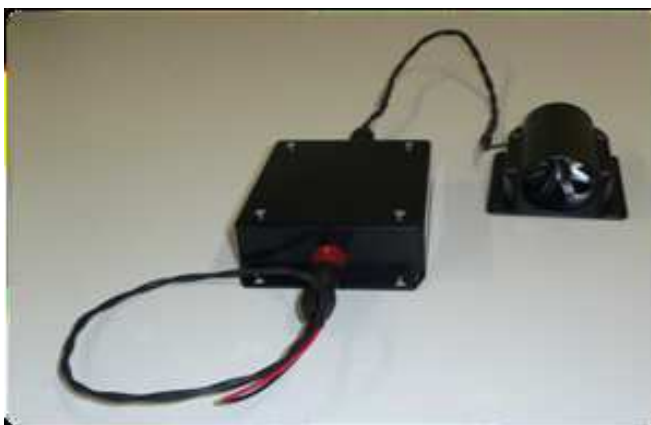
Fig. 16 The on-wing microturbine with its control electronics board
