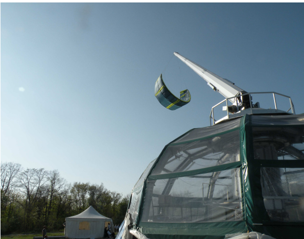
Fig. 14 optimized wing tested on the KiteGen generator
