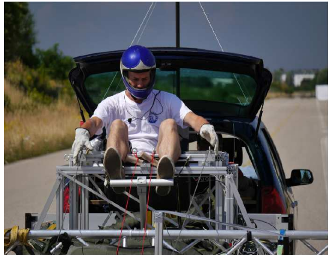
Fig. 13 The optimized wing preliminary performance test with a specially manufactured pilot testbench device
