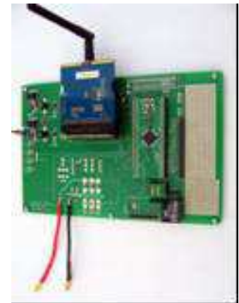
Fig. 15 The on wing electronic control board, with radio transmission device
