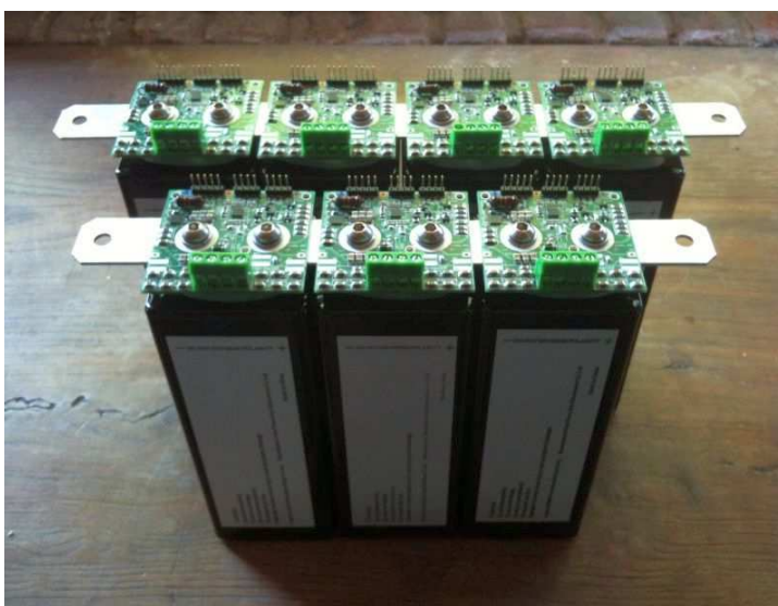
Fig. 6 Ultracapacitors with their specific charge control circuit
