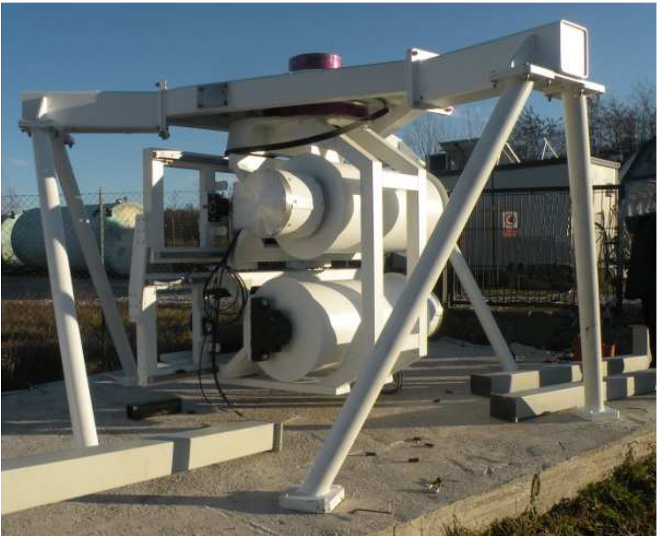
Fig. 1 The KSU base frame with alternators and drums
