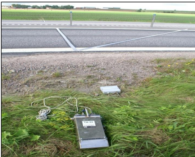
Photograph 2. Traffic analyser TA89 and charge amplifier. (Photo. Terence McGarvey)
