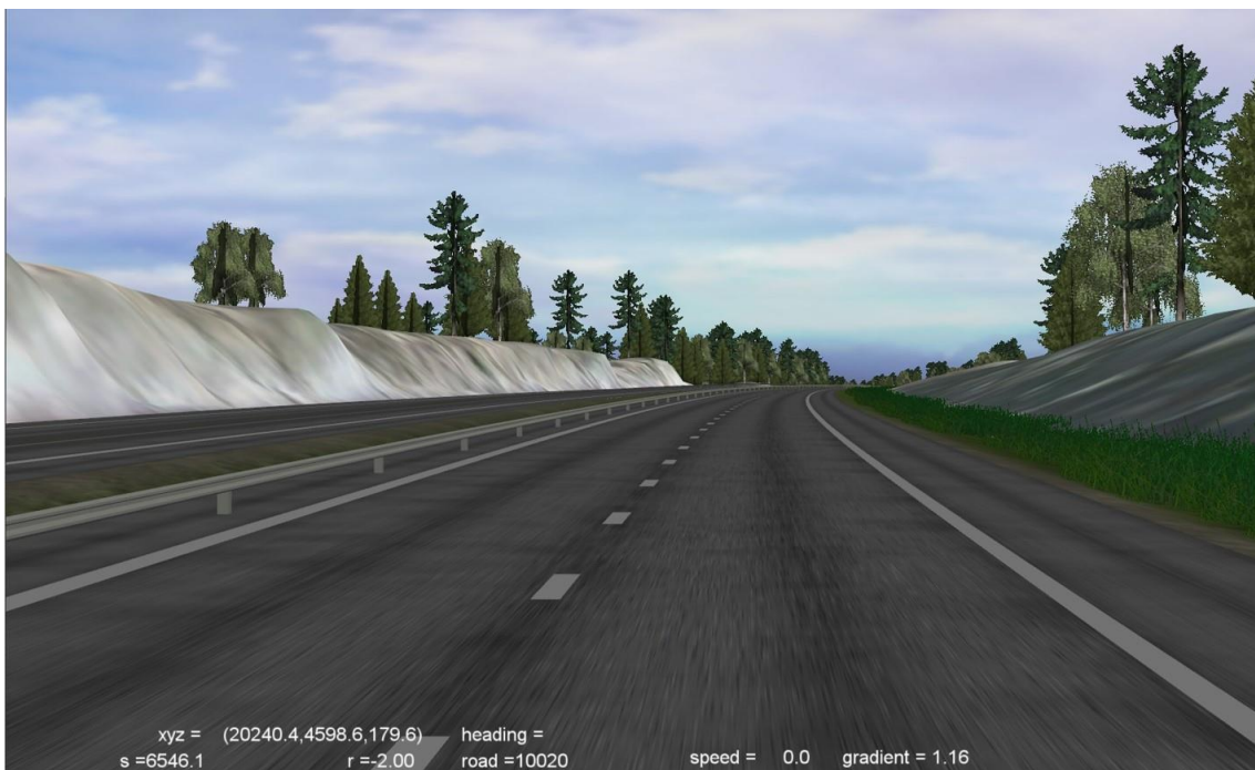
Figure 13. Picture of Road 40 after refinement. The more or less manual treatments following upon the automatic road generation consist of adding road embankment, vegetation, guard rails and special objects.
