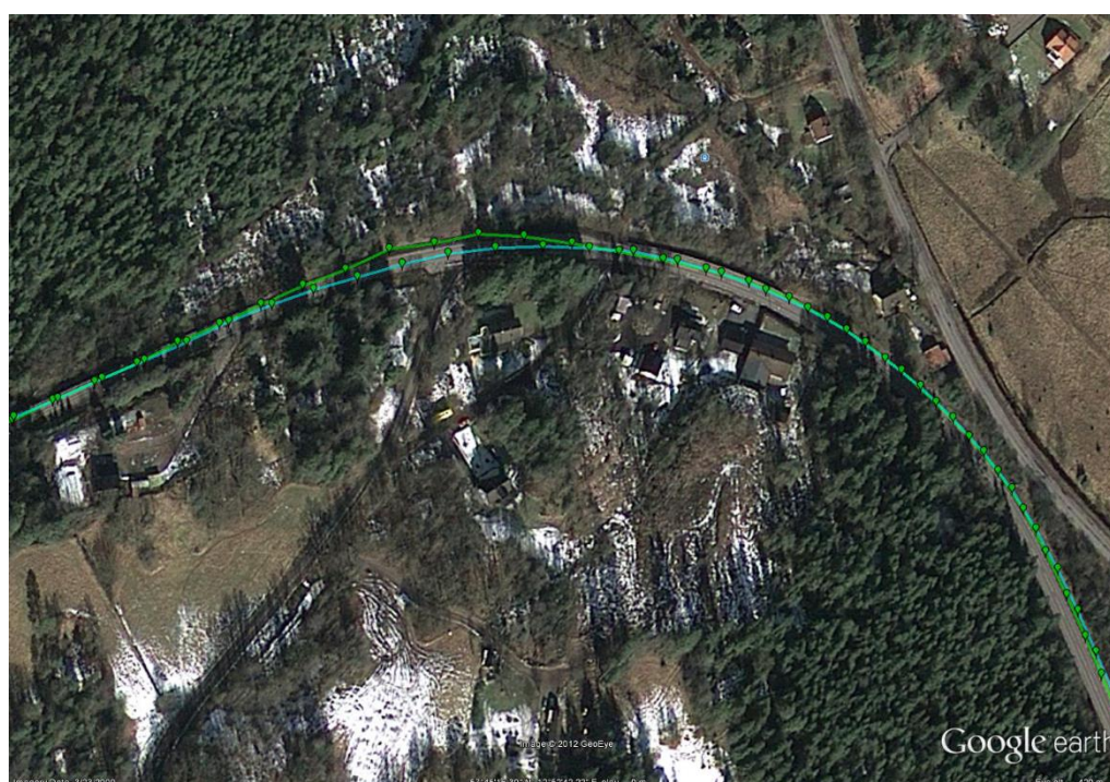
Figure 3. GPS measurements from the RST vehicle in two directions projected on a satellite photo in Google Maps.
