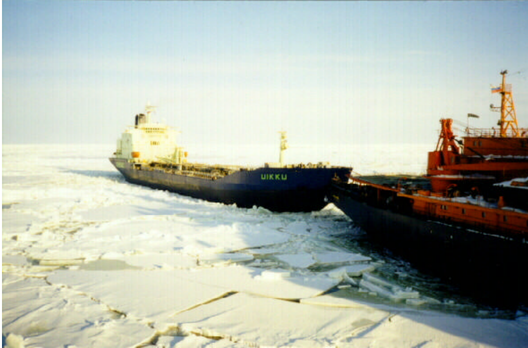
Figure 14 Towing of tanker Uikku by icebreaker Rossia in the Kara Sea
