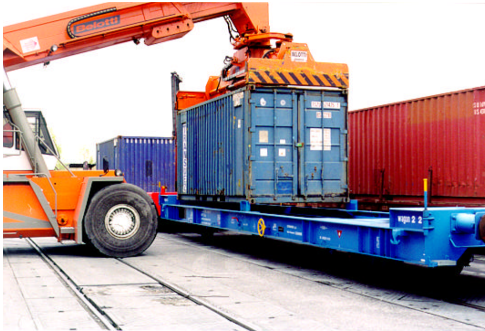
Fig. 4.9.4/2: Loading Wagon 222 with 20' Container by Reach Stacker
