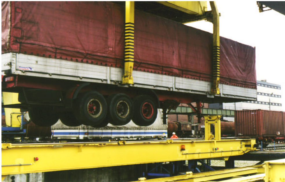
Fig. 4.8.5/2: Automated Unloading of a Semi-Trailer
