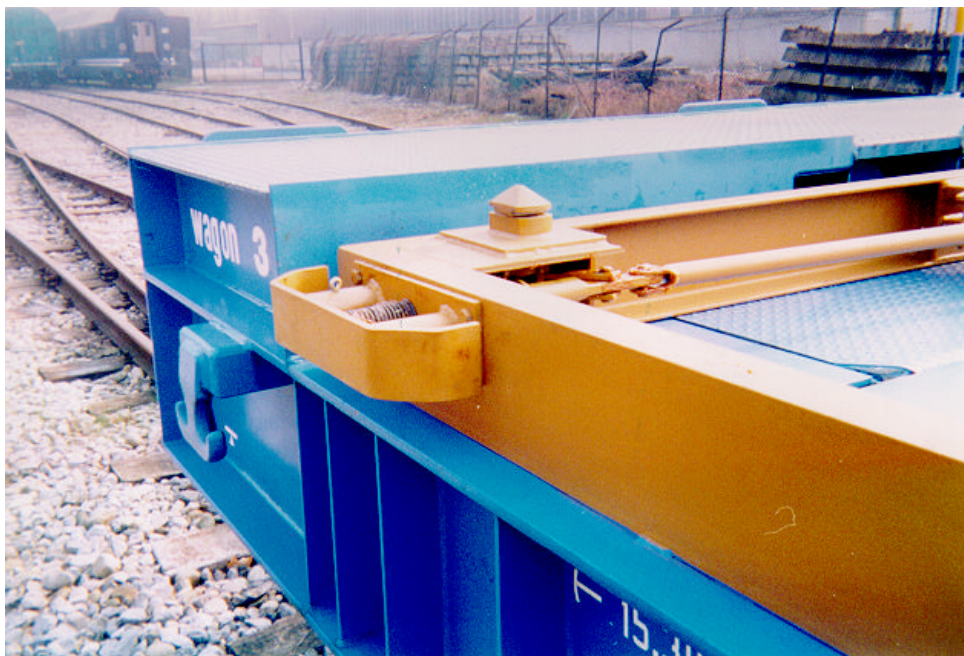
Fig. 4.9.3.2/6: Lower Twist Lock with Levers on Wagon 333
