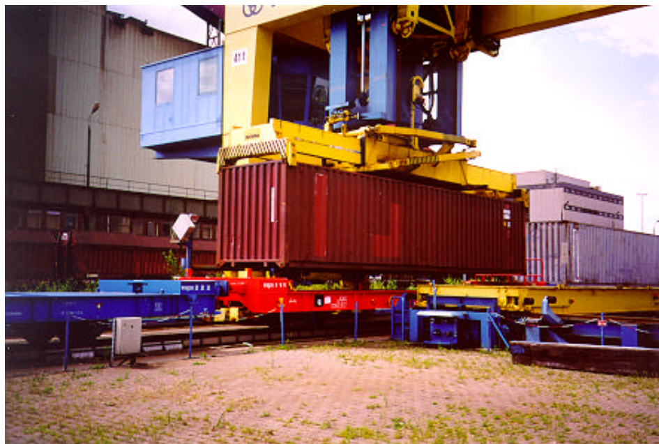
Fig. 4.9.5/2: Unloading Wagon 111 in Automated Terminal
