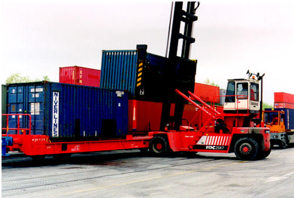
Fig. 4.9.4/1: Loading Wagon 111 with 20' Container by Fork Lift Truck
