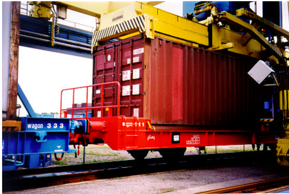
Fig. 4.9.5/1: Loading 40' Container on Wagon 111 in Automated Terminal
