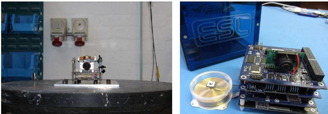
Figure 3: The prototype ADCS stack in vibration testing (left) and hardware-in-the-loop testing (right).
