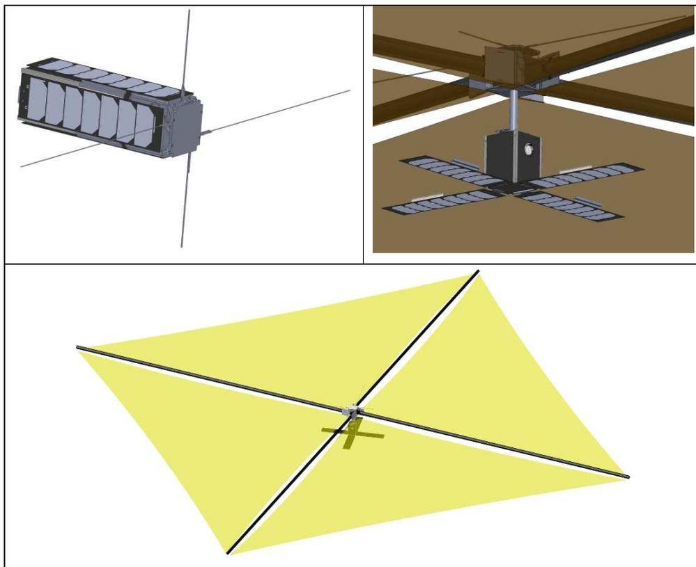
Figure 1: Three views of DeOrbitSail: before deployment, after deployment close-up, and after deployment from a distance.
