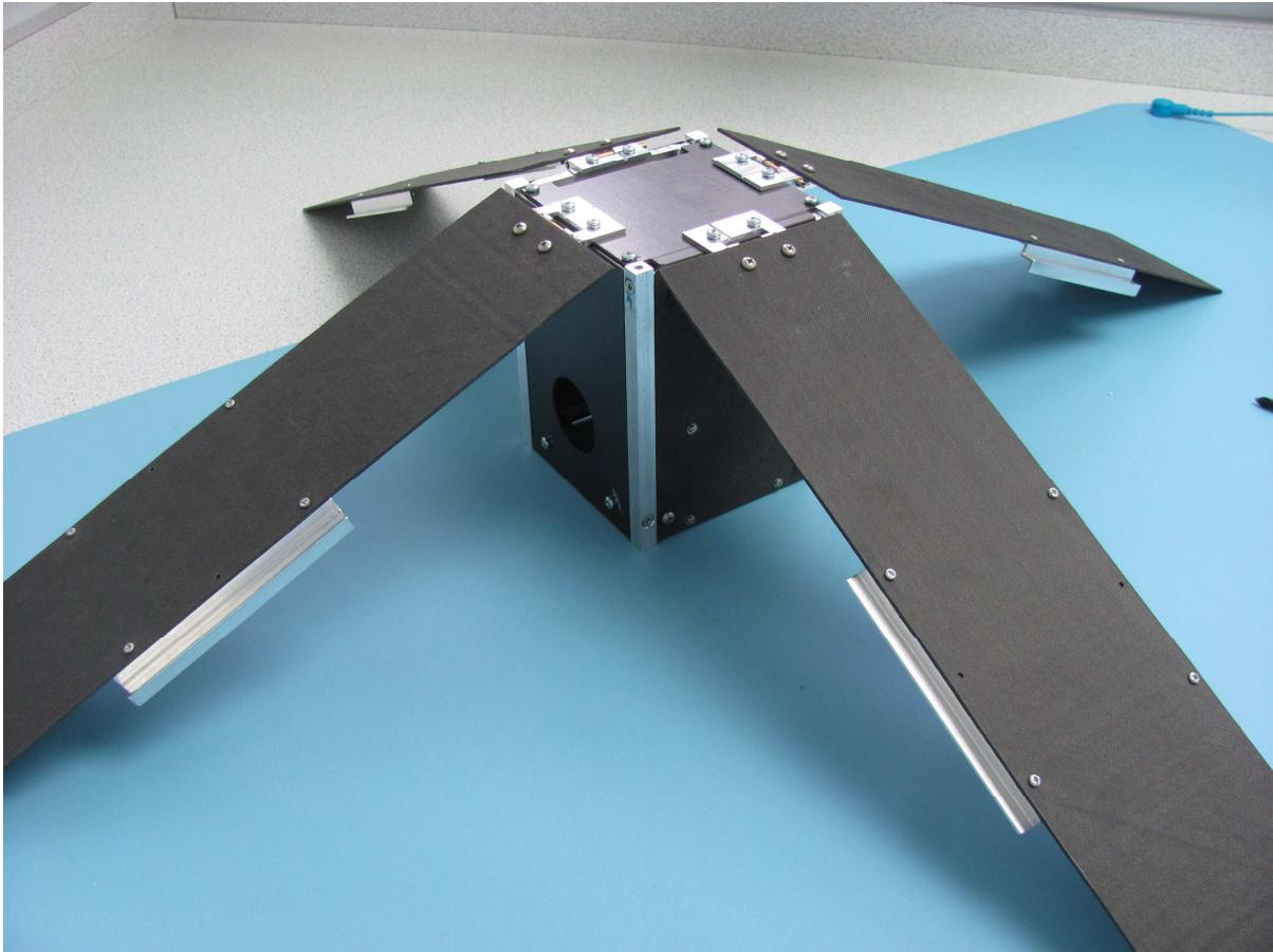
Figure 2: DeOrbitSail Qualification model: Assembled Chassis with solar panels .
