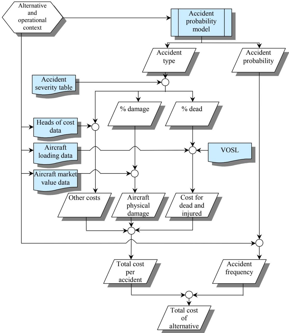
Fig 6: Accident cost calculation flowchart
