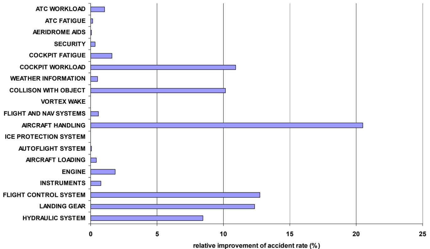
*Figure 2: Relative influence of the base nodes on the overall accident rate*
