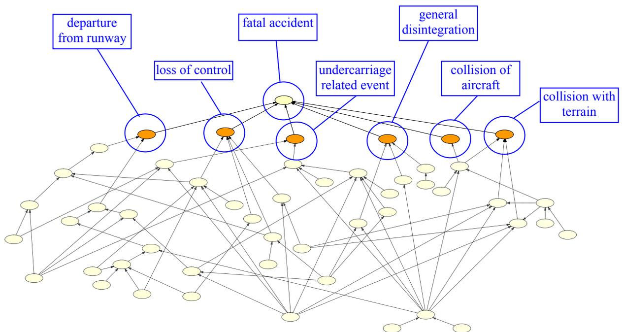
*Figure 8: Main accident types in the ASTER accident probability model*
