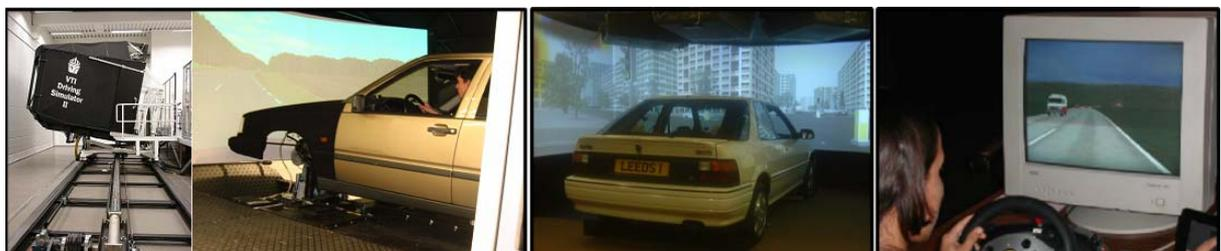
**Figure 5 – Moving base driving simulator (left), static driving simulator (centre) and laboratory set up (right)**
