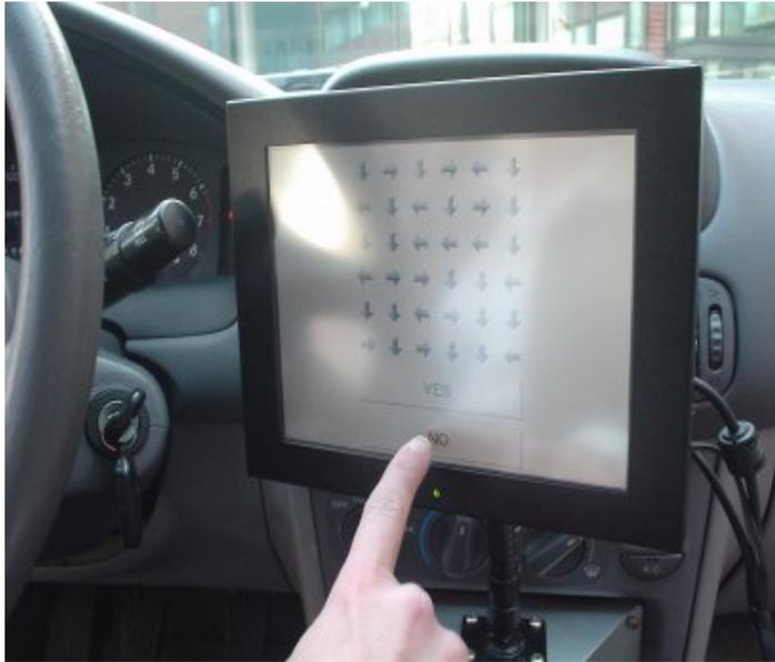
**Figure 3 – Visual S-IVIS in a car (Helsinki)**
