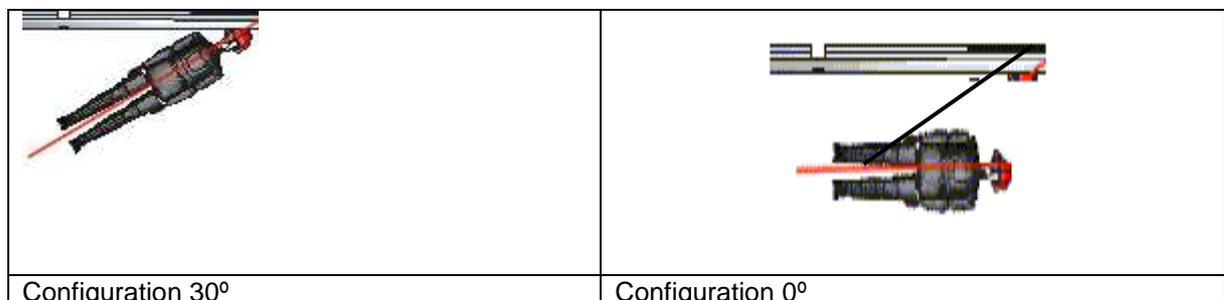
Figure 1: Impact configurations of the test proposed by LIER (France)
