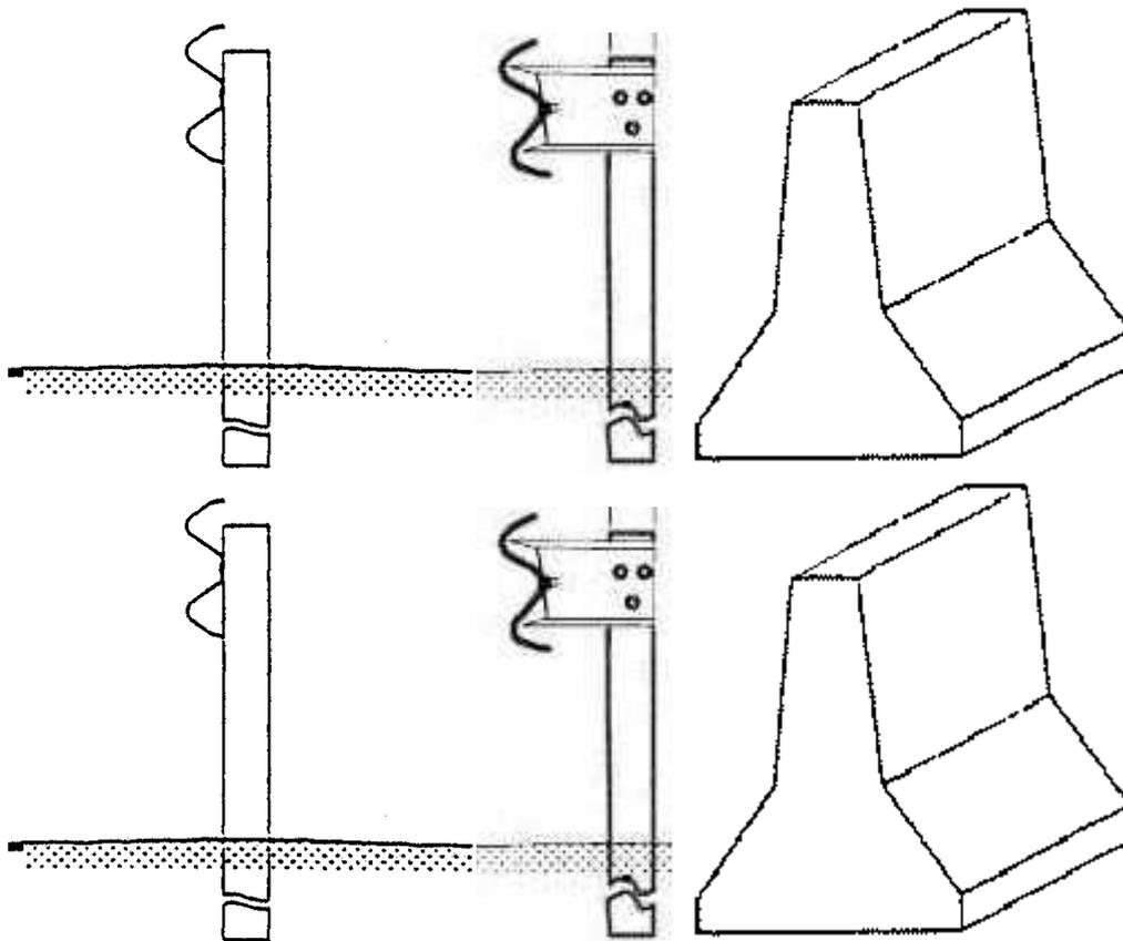
*Figure 6: Cross sections of simple guardrail, guardrail spacer-type, concrete barrier*
