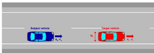
Regarding the straight road, the objective of the chosen scenario is to validate that the subject vehicle can detect and handle (warn, support, and/or intervene) a target vehicle in the same lane.
