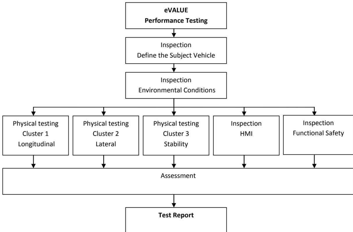
Figure 7 – The eVALUE performance testing process<sup>6</sup>
