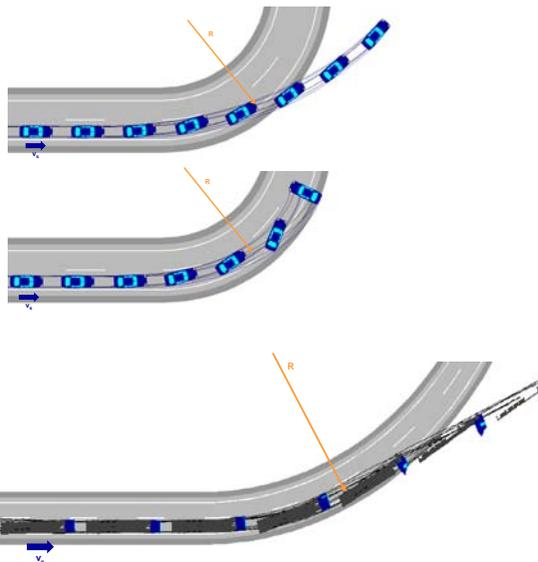
Evaluate the subject vehicle capability to avoid a loss of control as well as a lane/road departure in the case of approaching a curve too fast.
