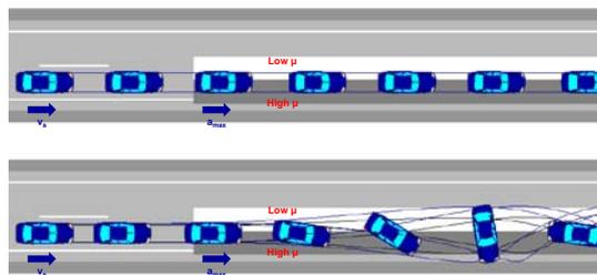
Emergency braking on a  $\mu$ -split, i.e. surfaces with different friction coefficients. Evaluate the subject vehicle capability to stop in a reasonable space keeping the desired driving direction while braking on asymmetric surface.
