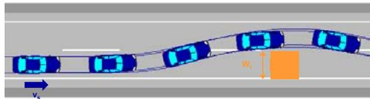
Evaluate the subject vehicle capability to avoid the loss of control in case of a sudden obstacle avoidance manoeuvre, followed by a come back to the original lane in order to avoid the collision with an incoming vehicle.
