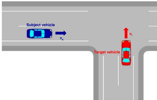
The objective of the third scenario is to validate that the subject vehicle can detect and handle (warn, support, and/or intervene) a target (e.g. other vehicle, pedestrians ...) which moves lateral to the subject vehicle.
