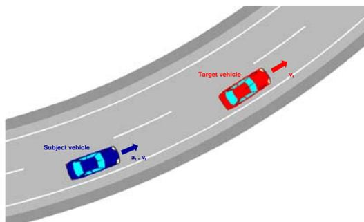
The same objective applies for the scenario for a curved road, i.e. validate that the subject vehicle can detect and handle (warn, support, and/or intervene) a target vehicle in the same lane on a curved road.
