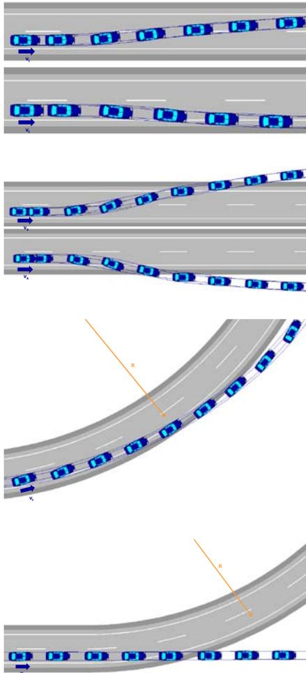
Meant to validate the subject vehicle capability to avoid involuntary (left/right) lane departure driving on a straight road. As a form of extension of the first scenario, the second is meant to validate the subject vehicle capability to avoid involuntary road departure driving on a straight road.
