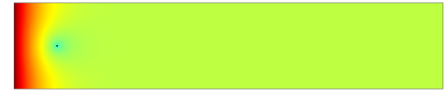
Top view pH map inside occluded cell
