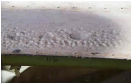
Fuselage showing damage to protective coating
