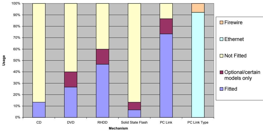
**Figure 21. Download mechanisms used by legacy VDR/S-VDR systems surveyed**
