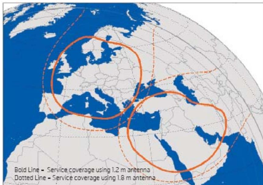
Figure 27 Telenor’s “DVB-RCS” service coverage (Courtesy of Telenor Satellite Services)
