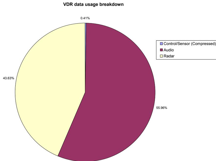
**Figure 3. Breakdown of the space usage of each type of VDR data with control/sensor data compressed**
