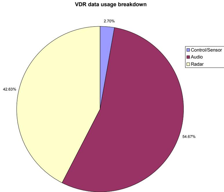
**Figure 1. Breakdown of the space usage of each type of VDR data**
