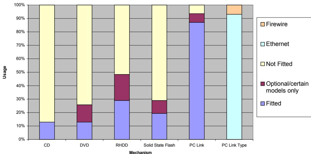
**Figure 17. Download mechanisms used by all VDR/S-VDR systems surveyed**
