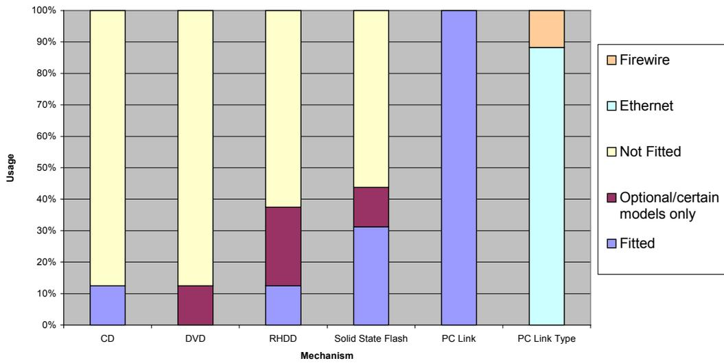
**Figure 19. Download mechanisms used by currently available VDR/S-VDR systems surveyed**
