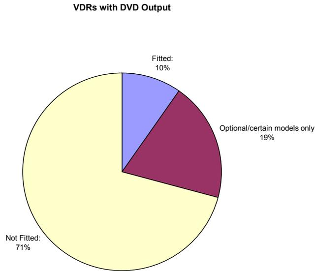
**Figure 7. The relative % of surveyed VDRs which are fitted with a DVD writer.**
