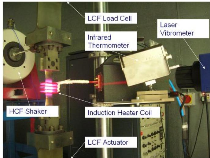
Figure 3 – Combined Cycle Fatigue rig
