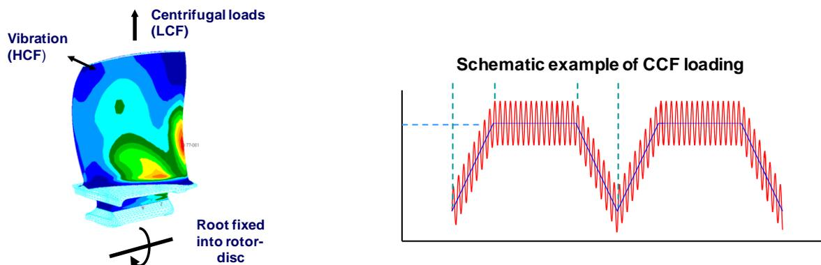
**Figure 1 – a) Schematic view showing Vibratory and Centrifugal Loads acting on a rotor blade (left) b) Schematic example of CCF loading (right)**
