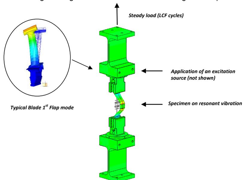
**Figure 2 - Schematic view showing a blade-like specimen test (right) simulating a rotor blade under resonant vibration of its first flexural mode (left)**
