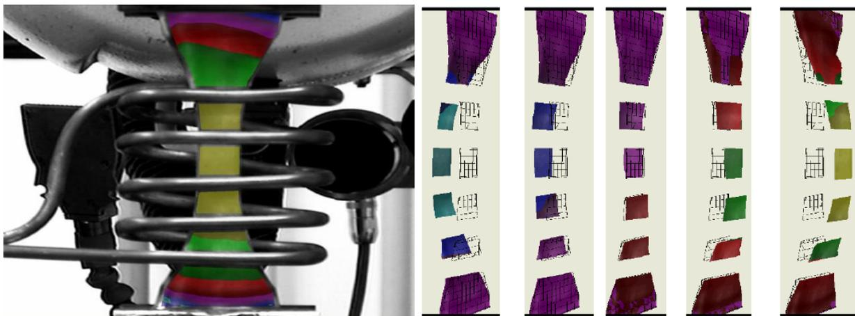
Figure 4 - Qualitative plots of the mode shape tested in one of the CCF rigs
