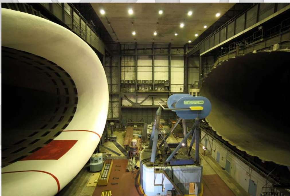
Setup of Smart Droop Nose in TsAGIs T101 wind tunnel (source: BockFilm)
