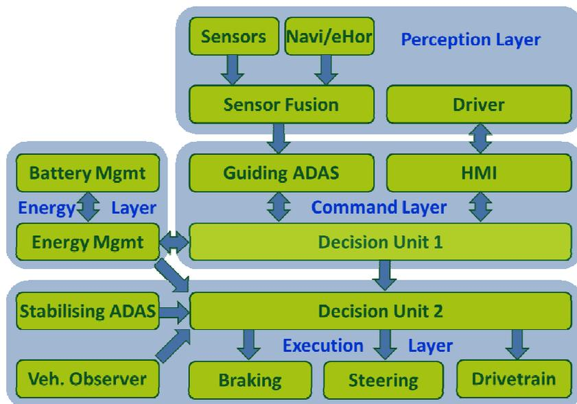
Top level functional architecture of the eFuture vehicle. ADAS stands for Advanced Driver Assistance Systems, HMI is the abbreviation for Human-Machine-Interface
