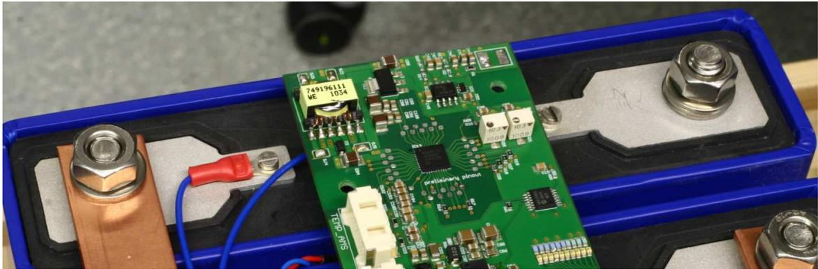
**Example of Battery Monitoring IC from autriamicrosystems (AS8505) evaluated by Fraunhofer IISB in the E3Car project**
