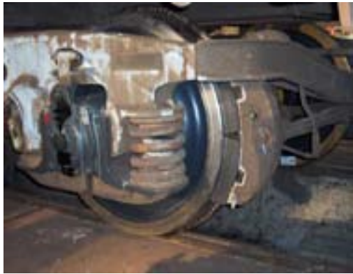
Figure 3.2. Picture of wagon retrofitted with k-blocks. Old wagons such as these are now as silent as modern passenger vehicles.
