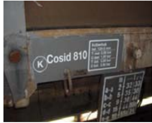
Figure 3.2. Picture of wagon retrofitted with k-blocks. Old wagons such as these are now as silent as modern passenger vehicles.
