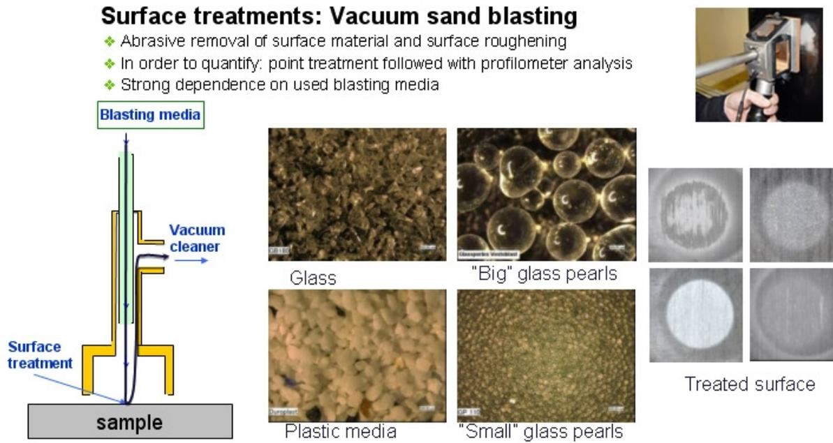
A surface pre-treatment with a vacuum sand blasting permits to replace the conventional manual grinding, improves bonding strength and permits to remove the eventual surface contamination. Its big advantage in respect to conventional sand blasting methods is the possibility to perform the treatments without the need for any special protective equipment. Thanks to the system design, blasting dust cannot escape even in case of leaks or other defects. The attractiveness to use it in
