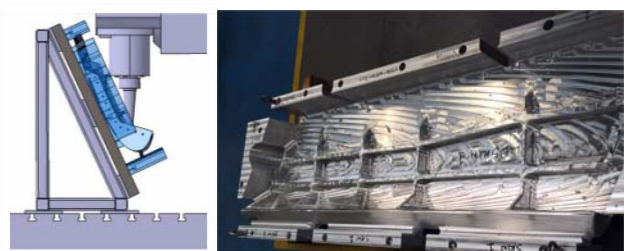
Figure 10: LE Section Machining Jig (Left) and LE Section Roughing Out (right)
