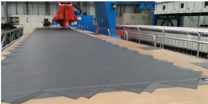
Figure 3: ATL at GKN Production Plant
