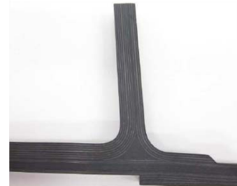
Figure 4: Cross Section Cut of Spar Cap showing the Pre-Cured Noodle
