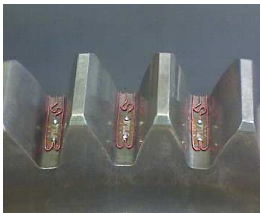
Figure 1: Instrumented gear with strain gauges
