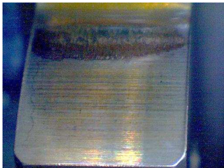
Figure 7: Scuffing on the tooth dedendum of a tested gear
