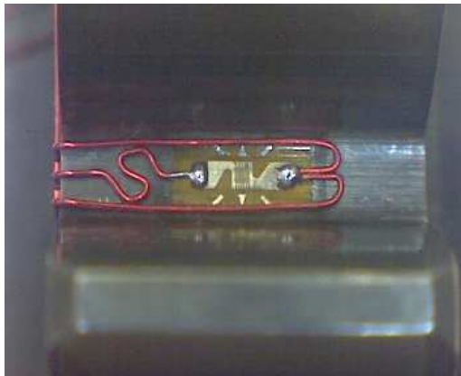
Figure 2: Detail of an instrumented gear tooth root fillet
