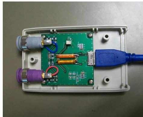
1kV Neel Effect® Voltage transducer
