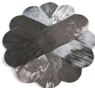
Figure 4. FPP carbon fibre reinforcement rosette (EADS-IWG)
