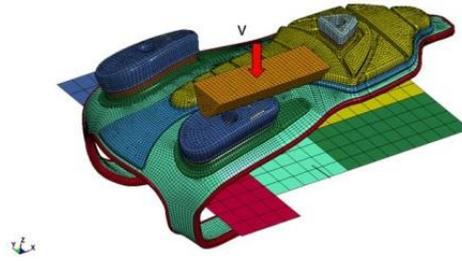
Fig. 1. Simulation of Kid-Shell protection test.
