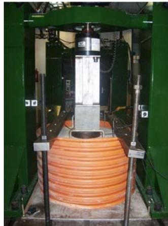
Fig. 11. Cyclic loading tests carried out on NEOBALLAST and conventional ballast.
