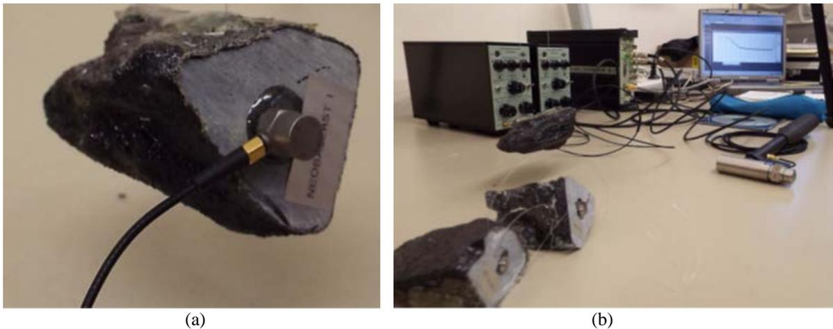
Fig. 9 (a) Accelerometer inside a NEOBALLAST aggregate; (b) Equipment required for the vibration mitigation test.
