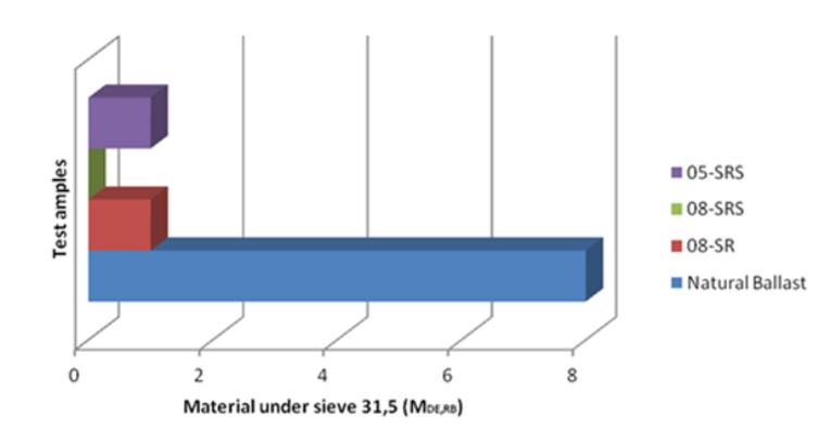
Fig. 6. Results of Micro-Deval tests for NEOBALLAST (four configurations) and natural ballast.
