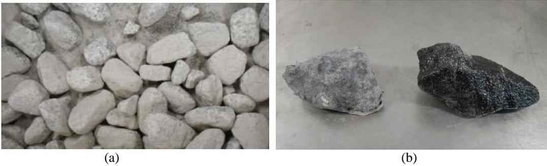
Fig. 5. (a) Natural ballast after the LA test; (b) Two samples of NEOBALLAST after the tests.
