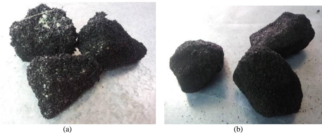
Fig. 2. (a) NEOBALLAST coating with large rubber particles; (b) NEOBALLAST coating with small rubber particles.
