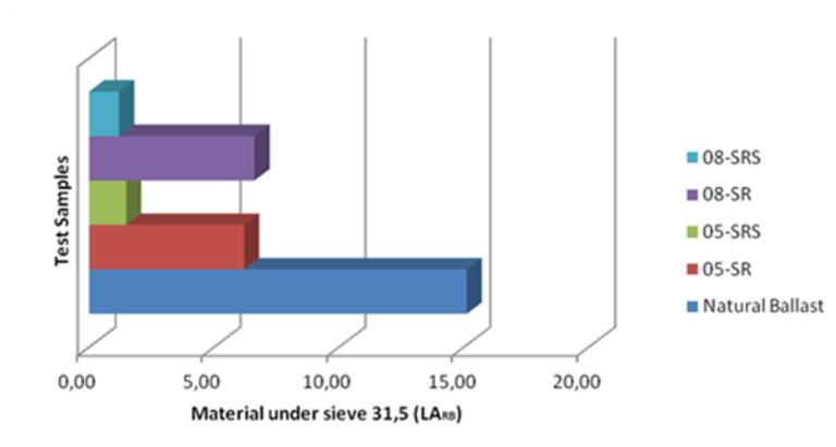
Fig. 4. Results of LA test for NEOBALLAST and granite ballast aggregates.
