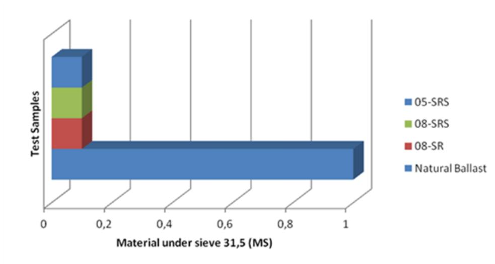
Fig. 8. Magnesium sulphate test results for NEOBALLAST and natural ballast aggregates.
