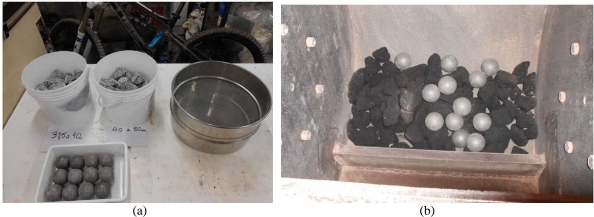
Fig. 3. (a) Los Angeles test material; (b) NEOBALLAST sample inside the drum.
