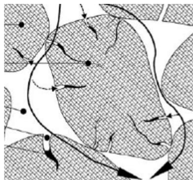
Fig. 7. Scheme showing how water transport occurs within the rockfill specimen.
