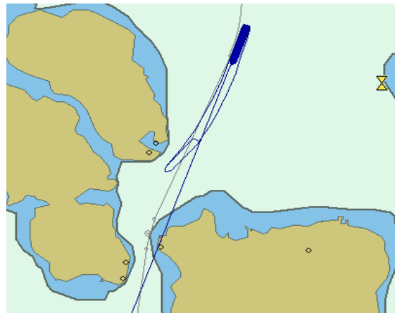
Figure 9: True scale ship symbol on electronic chart display showing heading marker and one-minute path prediction
