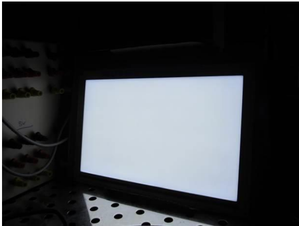
Figure 2.5.3.2 DHA in the HALT test chamber
