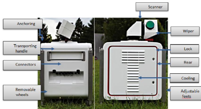
Figure 2 – Picture of the UFO Lidar with a High Power laser source (casing and mechanical were reused from an existing equipment)
