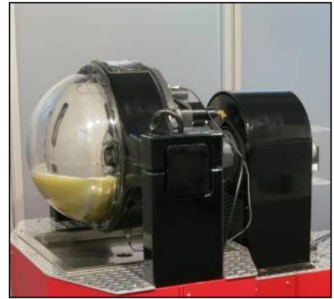
Fig. 2 - Demo-bench with oil level control system in the differential.
