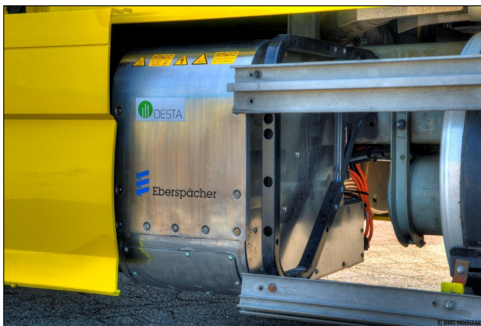
Figure 39: The SOFC APU installed on the chassis frame of the vehicle
