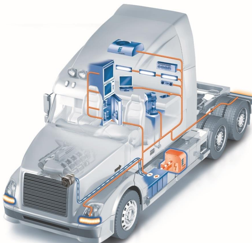
Figure 32: SOFC APU concept in a Truck (Eberspächer)
