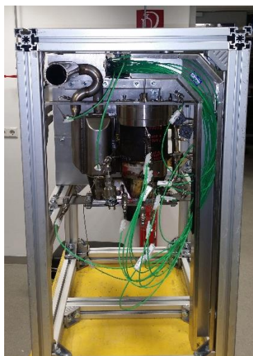
Figure 21: Re-Designed two-stack APU system during assembly
