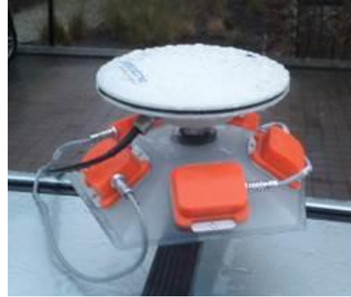
Figure 48 Measurement campaign setup with five MTi xSense inertial sensors and Septentrio Asterix receivers
