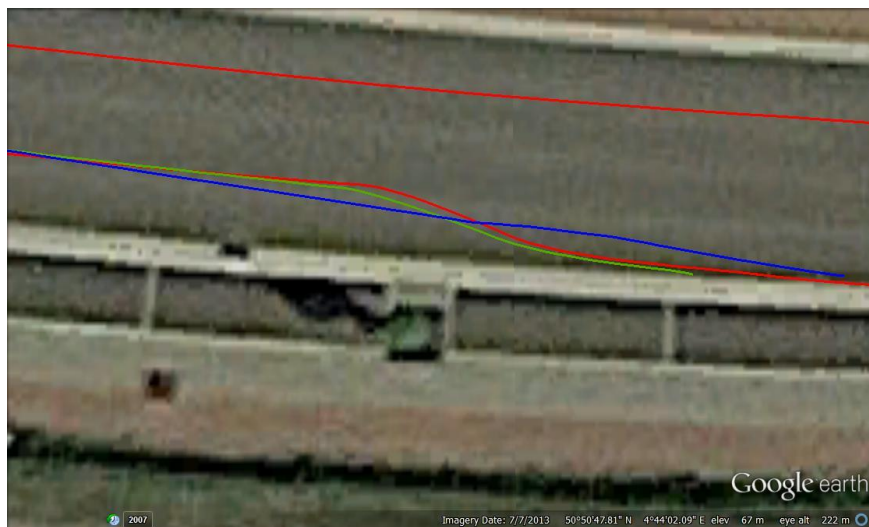
Figure 46 - Comparison of the Reference solution (red), unadjusted Vision solution (blue) and the yaw adjusted solution (green)
