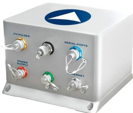
Figure 42 The ATLANS-C implementation (based on SSN Ax3 and iXBLUE IMU50)
