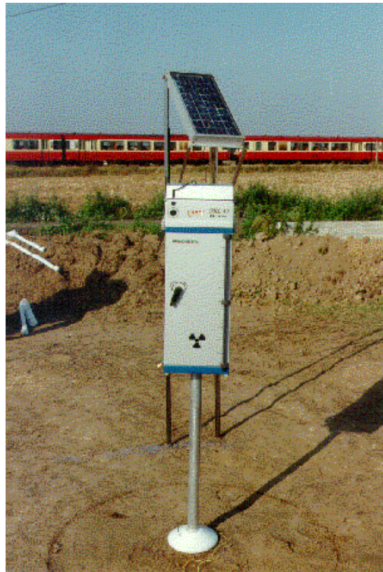
Figure 6.5 Neutron humidimeter used in the field (Lille – France)
