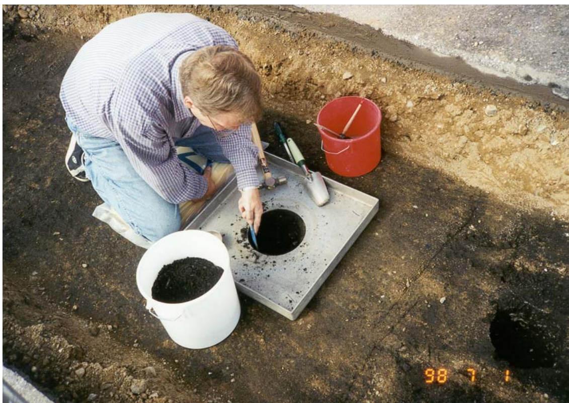
Figure 7.2 Measurement of field density at the site (Sand replacement method)
