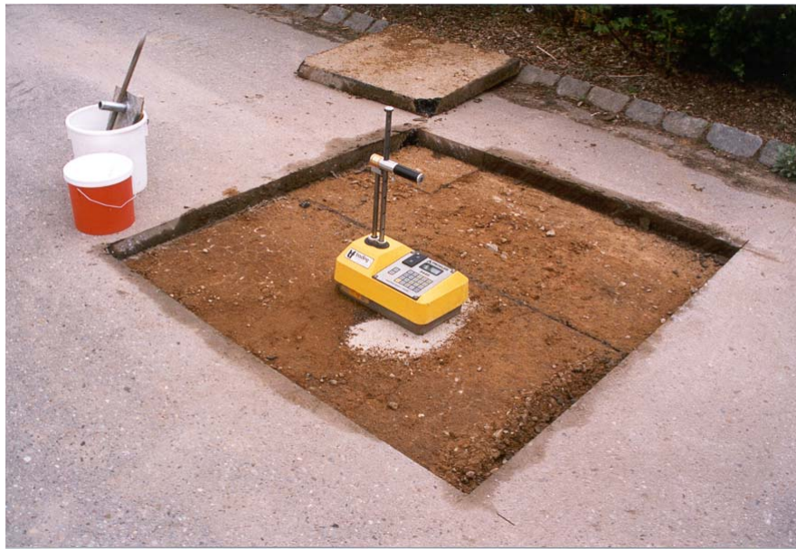
Figure 7.1 Measurement of field density at the site (nuclear gauge method)
