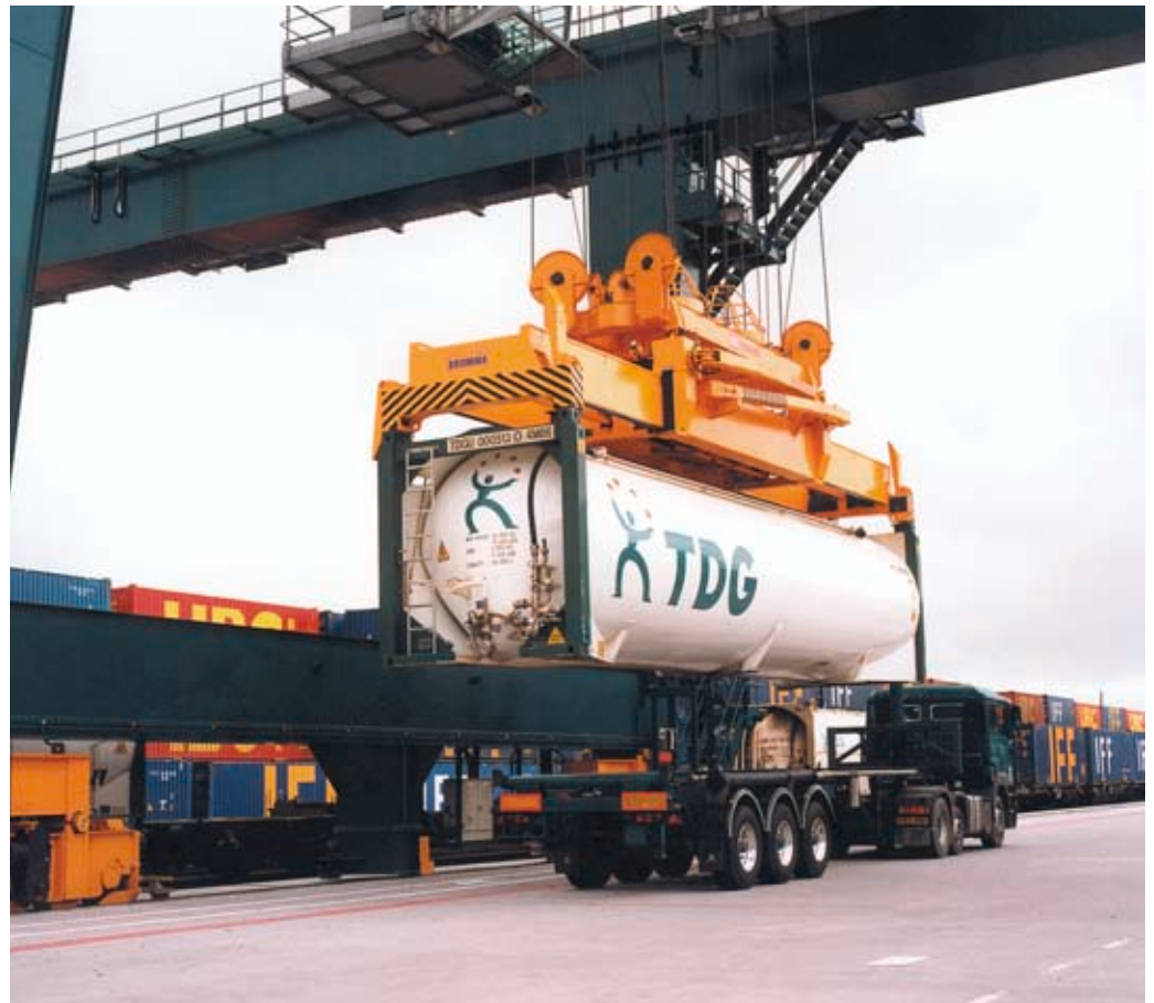
Combi tank being transferred from rail onto road vehicle for onward movement
