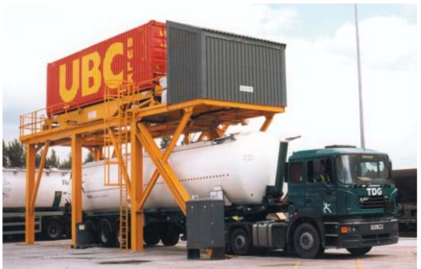
Decanting UBC box into TDG road barrel at Grangemouth Terminal
