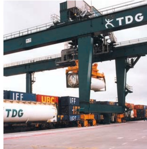
Crane lifting TDG combi tank
