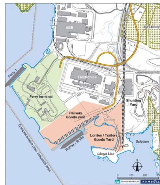
Port area with planned marshalling yard.
