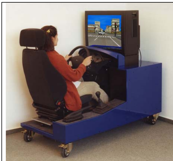
Figure 5: The low-cost simulator layout with a single monitor.
