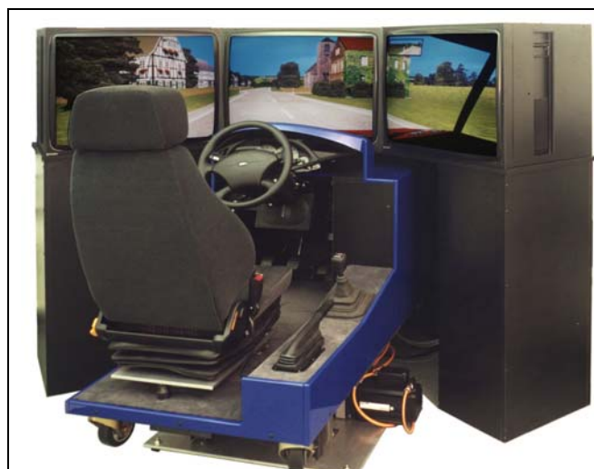
Figure 7: The mean-cost simulator layout with three single monitors.
