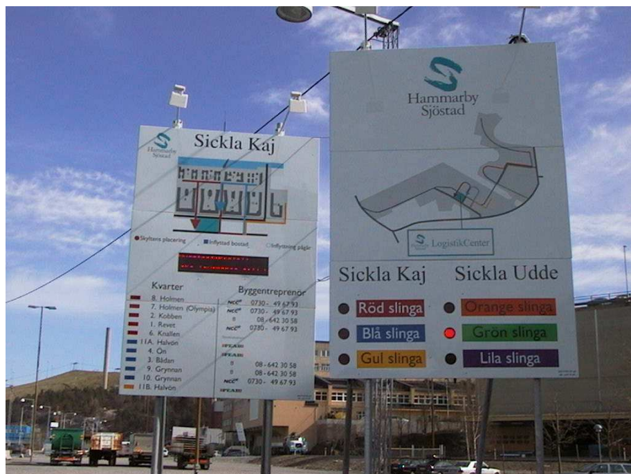
Figure 84: Truck guidance by smart traffic signs [Brisvall 2002]
