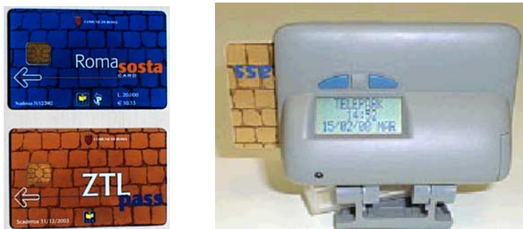
Figure 58: Smart cards and On-Board-Unit (OBU) [Tomassini 2001]
