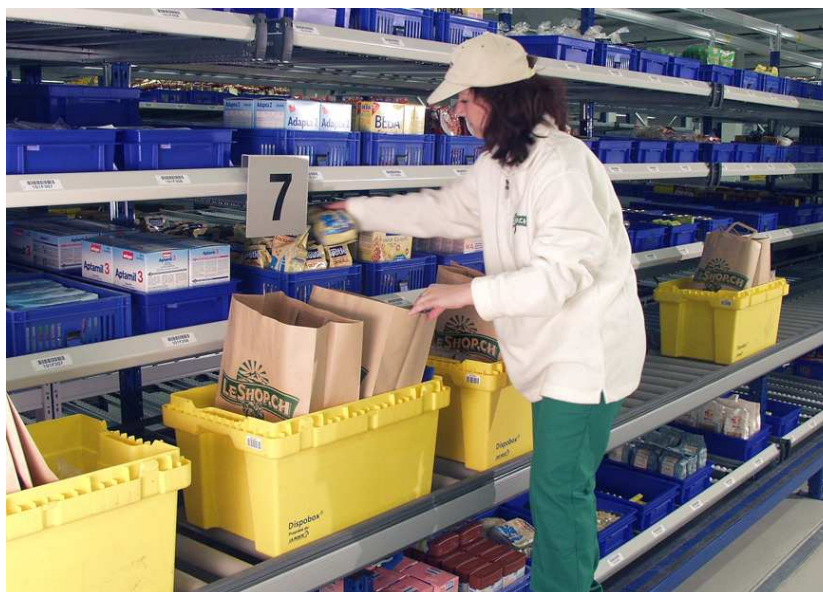
Figure 36: Picking process using conveyor belts in LeShop's dedicated warehouse [www.leshop.ch]
